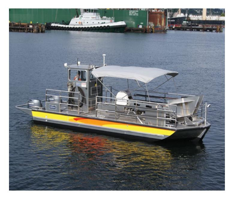
The 31ft Kvichak/MARCO Filterbelt boat is a rapid response skimming vessel that can operate in protected waters such as ports, harbors and inland environments. The lightweight construction allows this boat to rapidly arrive on scene and immediately start cleanup operations. The boat incorporates an advancing filter belt skimmer that enables the boat to skim oil while going through the water with high efficiency.
