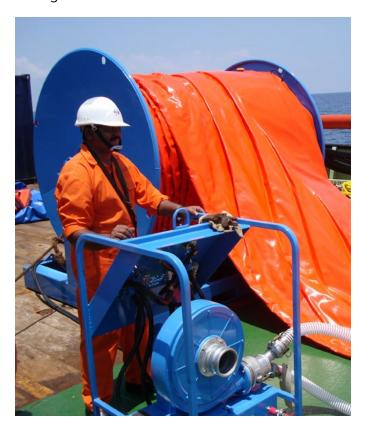
Elastec offers a full range of boom reels that can be delivered for all sizes of AirMax boom. These reels are available mounted on trailers or in storage containers. We also offer a full range of boom accessories including blowers, bridles, anchor sets, boom lights, choice of connectors, and tidal compensators. AirMax is available in six sizes. The size required will depend on the sea conditions or water body where the boom will be deployed.
