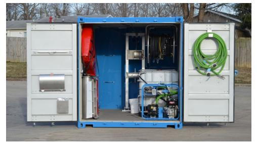
As an option we can provide the system mounted inside a 10ft container, once secured to the deck the container provides the mounting point for the Tow Tower.
