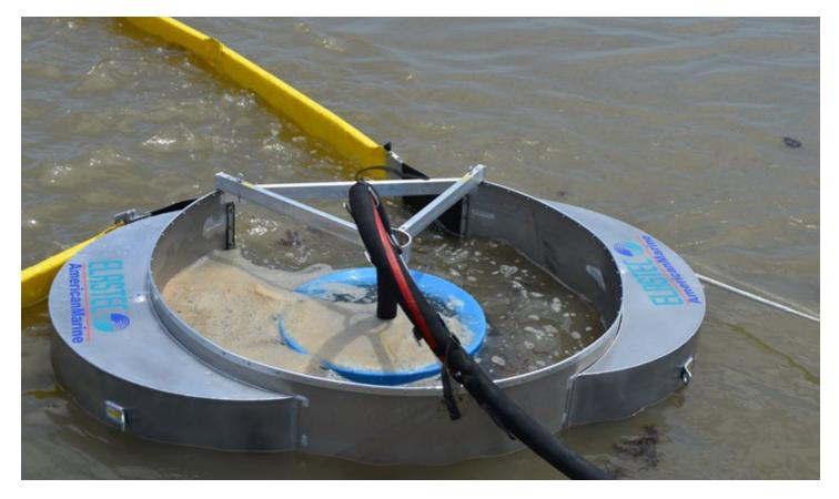
The Circus Skimmer is an in-line oil skimmer that is coupled with river boom and harnesses water flow to separate the oil and water. The skimmer has a circular chamber that accumulates the oil and allows the water to exit the bottom. This skimmer is ideal for calm river conditions. Tested at Ohmsett (an independent test facility) it was able to recover 90% of oil at 2 knots.
