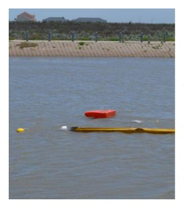
Rotation of the oil/water is generated by the river current. The circular flow in the chamber is created as the water entering the chamber is balanced by a corresponding flow exiting beneath the skimmer.
