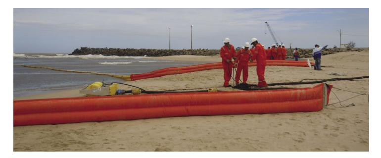
**ELASTEC TundraGuard** oil spill containment boom is effective in swamps, marshes and wetlands. It is a special purpose lightweight boom for use in shallow, calm water environments where the water level may fluctuate and cause conventional booms to leak or fail due to grounding.
