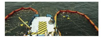
**ELASTEC RubberMax V-Sweep** is an inflatable rubber boom system for sweeping oil with a single vessel. An optional outrigger arm holds one end of the sweep open in a side sweep arrangement. The boom geometry is held in a V configuration to form a pocket of oil that can be recovered by most oil skimmers.
