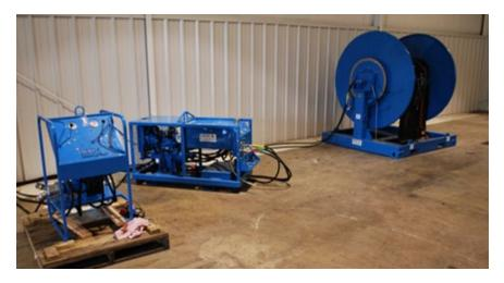
Note: The Power Pack is typically ordered with a Control Stand for operation of speed and direction of steel boom reels. One stand may be used for multiple reels. The control stand incorporates a hydraulic driven High Output Air Blower and boom reel/blower controls. The blower can rapidly inflate boom .
