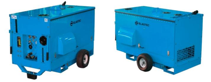
The D23S Diesel Hydraulic Power Unit is mounted on a rugged, aluminum base frame that contains welded forklift pockets and a lifting configuration to facilitate shipping and positioning. It features foldable handles to assist mobility by one person. It can operate in environments from -20° to 120° F (-6° to 49° C). This power unit was design for ruggedness, reliability, quiet operation, small size and ease of maintenance.
