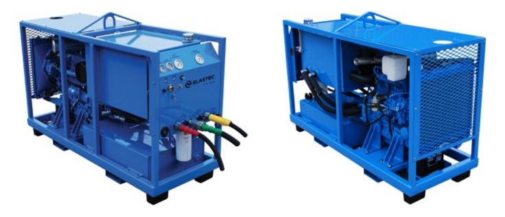
The D34 is a diesel driven hydraulic power pack with two variable flow hydraulic circuits. Driven by a powerful 43hp / 36kW water-cooled diesel engine driving twin fixed displacement hydraulic pumps, mounted in painted steel frame. Fork lift pockets, central lift point, hydraulic oil and fuel tanks are all incorporated in this compact unit. Twin hydraulic flow controls, gauges and stainless steel hydraulic couplings. Spin on return filter, fluid level and temp gauges, tank top filler/strainer.
