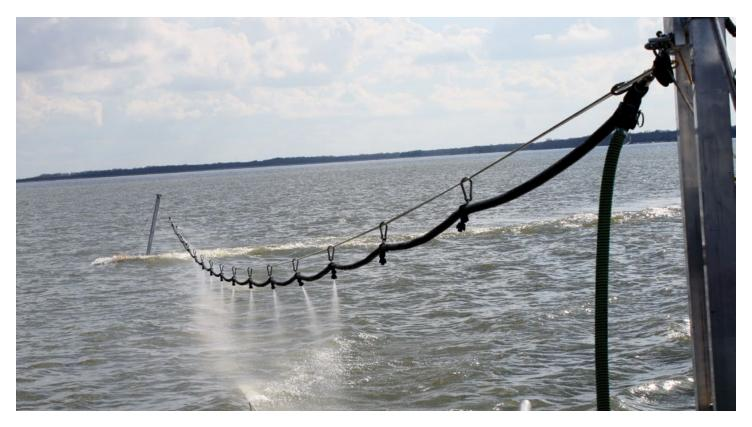
The **ELASTEC BoomVane™ Spray** system can be deployed from small service vessels, such as coastal fishing boats, pilot and work boats, for dispersant application on marine oil spills. The 1m BoomVane allows for a wider spray width (65 ft / 20 m) than conventional arm systems.
