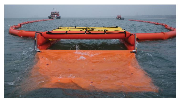
**ELASTEC NeatSweep**® is a precision oil spill dispersant application system that provides a large encounter rate for oil spilled on water. The dispersant pump automatically detects the speed of the towing vessel and self-adjusts the spraying rate according to pre-set parameters. A mixing panel is towed behind the dispersant application zone (DAZ) to help mix the oil spill dispersant with the oil on the water's surface.
