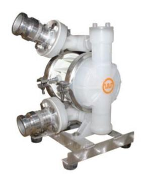
Elastec offers a 1 inch diaphragm pump with our drum skimmers. Diaphragm pumps can self-prime, do not typically emulsify recovered oil and can run dry. They are therefore a good match for an oil skimmer.
