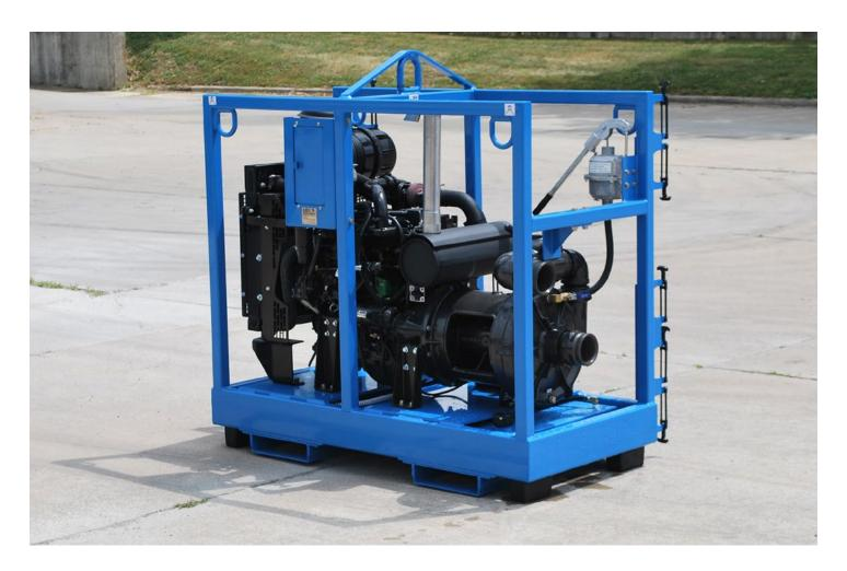
The E600 is a diesel driven high flow water pump that can be used for a variety of roles including fire fighting, water transfer, dewatering and liquid transfer. Mounted in a robust steel cage frame with fork pockets, central lift point and rubber mounts, it is offered with a choice of diesel engines.
