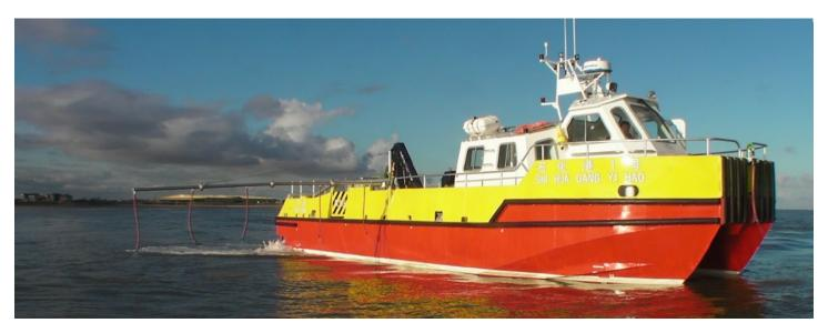
ElaSpray is a portable dispersant spraying system for use at harbors and offshore oil spill response operations. The system is designed for easy installation on tugboats, offshore supply vessels or other types of vessels. The system contains a compact diesel engine driven pump for spraying dilute or neat dispersant. A set of two marine grade aluminum spray arms are mounted on the supporting post and secured by the topping wires. Each standard spray arm is mounted with 5 spray nozzles.
