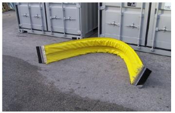
FlexiBelt is a unique spring loaded floating containment boom designed to be used by ships during refueling and product transfer operations. It will ride up and down against the ships' hull and seawall, automatically adjusting to the changing distances and waterline. Typically, two FlexiBelts are deployed with one upstream and one downstream (facing in opposite directions).
