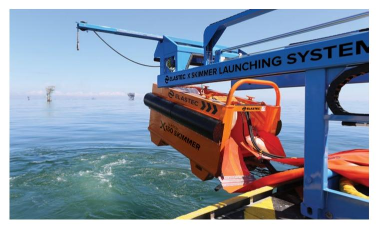
The **ELASTEC X150** is an advancing Grooved Disc skimmer that features the breakthrough oil skimming technology of our 64-disc prototype that won the Wendy Schmidt Oil Cleanup X CHALLENGE by recovering 4,670 gallons of oil per minute. The **ELASTEC X150 Skimmer Launching System** combines the X150 Grooved Disc Skimmer, power pack, boom reel, hoses and BoomVane<sup>™</sup> and is packaged to fit into a 20 ft container for rapid global shipment.
