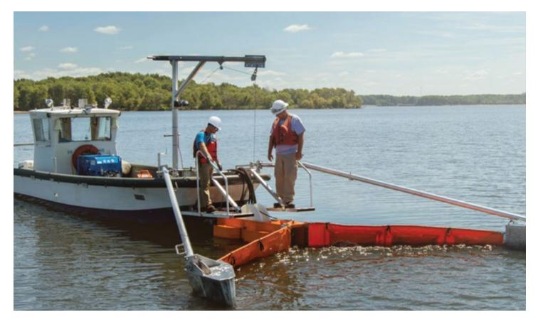
The **ELASTEC X30 Grooved Disc Skimmer** features twin discs in a module that can be incorporated into a bow or over-theside sweep system. Skimmed oil may be contained in on-board tanks or towed in an ELASTEC Towable Bladder. The X30 has been validated at Ohmsett.
