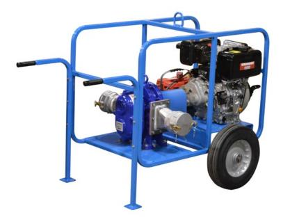
The Elastec Lobe pump is a heavy duty diesel driven pump set, the lobe pump is capable of handling solids and viscous materials. For industrial or oil spill applications up to for product transfer such as filling and emptying trucks and transferring slurry between pits. Matched to an electric start 9hp / 6.7kW diesel engine the pump can deliver up to 159 gpm / 36 m3/h @ 58 psi / 4 bar.
