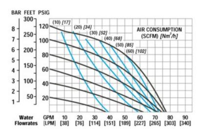
Elastec offers a 11/2" inch diaphragm pump with our drum skimmers. Diaphragm pumps can self-prime, do not typically emulsify recovered oil and can run dry. They are therefore a good match for an oil skimmer. The M4 pump is supplied with Aluminum, Cast Iron or Stainless body according to the application. Buna, Neoprene, Viton or PTFE Diaphragms & Ball Valves are available.
