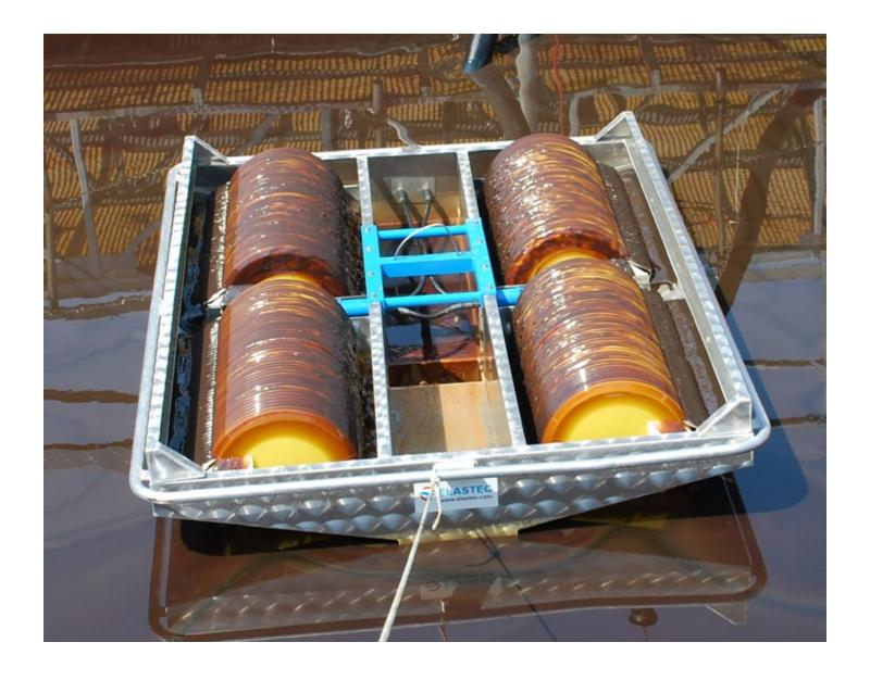
Drive is provided for the drums by a pair of centrally mounted gearboxes (provides even weight distribution), these gearboxes provide the torque necessary to turn the drums in heavy oils as well as allowing for fine control of the drum speed. The drum shafts are supported by self-aligning bearings. This is all mounted in a lightweight anodized marine grade aluminum frame with open and steeply inclined pathways that direct recovered oil to where a high capacity salvage pump is located.
