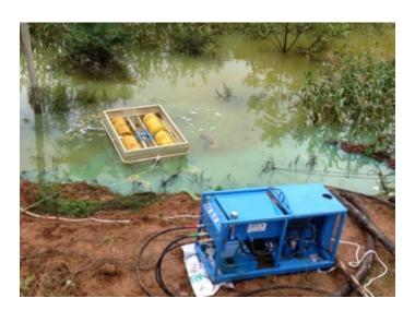
The ELASTEC Magnum 200 is another well proven drum skimmer from Elastec. It is suitable for both oil spill response in inland, harbor, coastal and open water. The lightweight design combined with the stability and high buoyancy provided by the four drums enable the Magnum 200 to be used in such a wide variety of environments.
