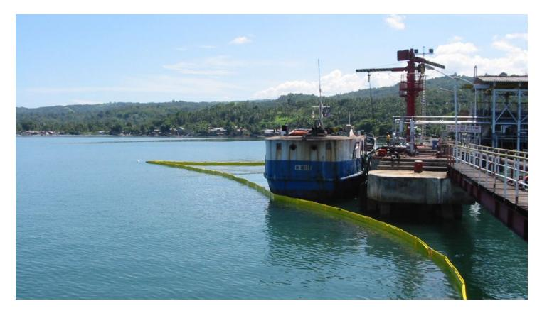
Elastec manufactures a line of fence boom with added tension members combined with solid foam flotation. This oil and debris barrier is typically used for rapid deployment in ports and harbors for surrounding vessels or protecting resources. The construction employs top and bottom tension members (cable on top and chain on bottom). Even if the fabric is damaged these members will hold the boom together.
