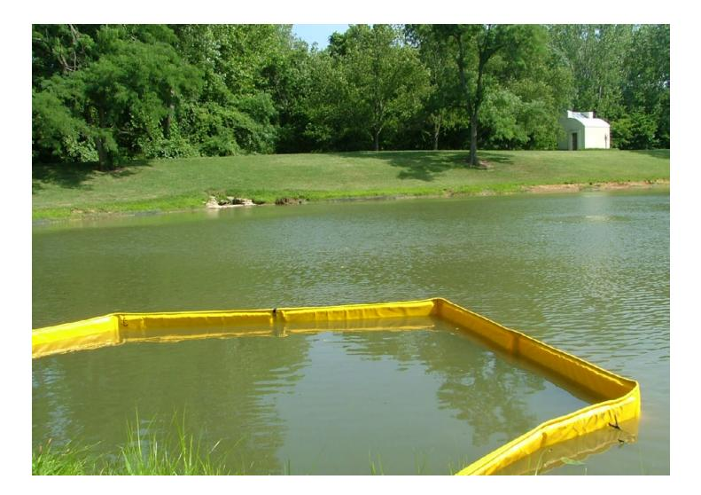
The construction of these booms does not use sewing that would allow water to enter the float chambers, instead its' float pockets are fully welded for a water tight seal. The floats are closed cell ensuring that they will not take up water and provides strength to be wound on a reel without deformation.
