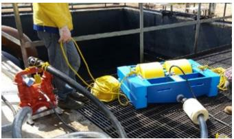
Elastec pneumatic skimmers are fitted with air motors that conform to EC Directive 94/9EC (ATEX 100a) for zones 1 and 2 (Group II, category 2, Gas and Dust Atmospheres) and a maximum surface temperature of 275 F / 135 C.
