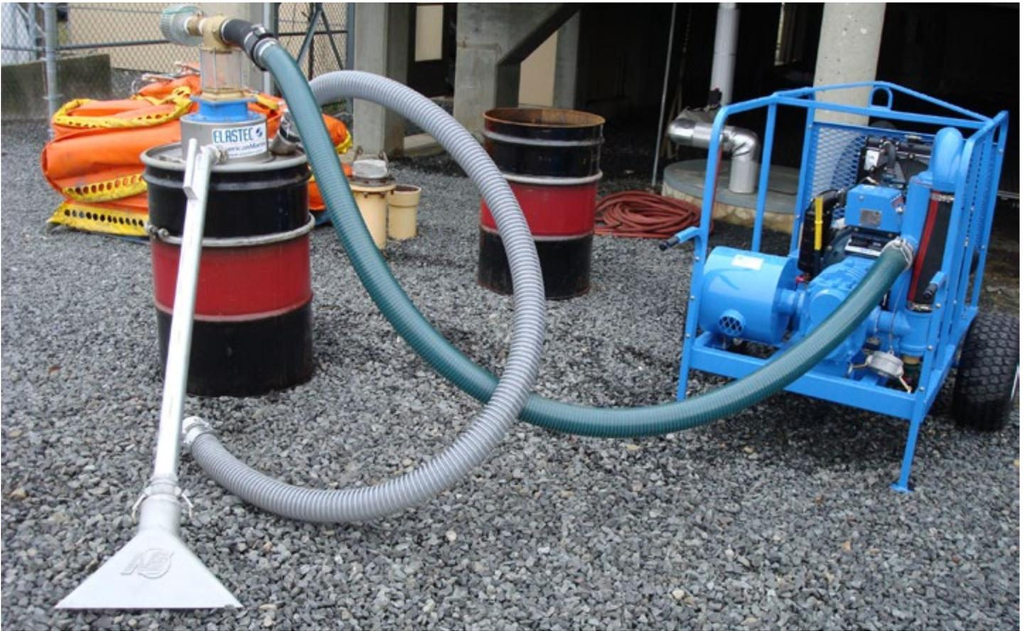
The ELASTEC MiniVac II is a high powered vacuum system that offers powerful vacuum abilities and easy mobility. The MiniVac II can go places that are simply not accessible by vacuum trucks. The wheels and handles can be removed so that the unit will sit in the bed of trucks etc.
