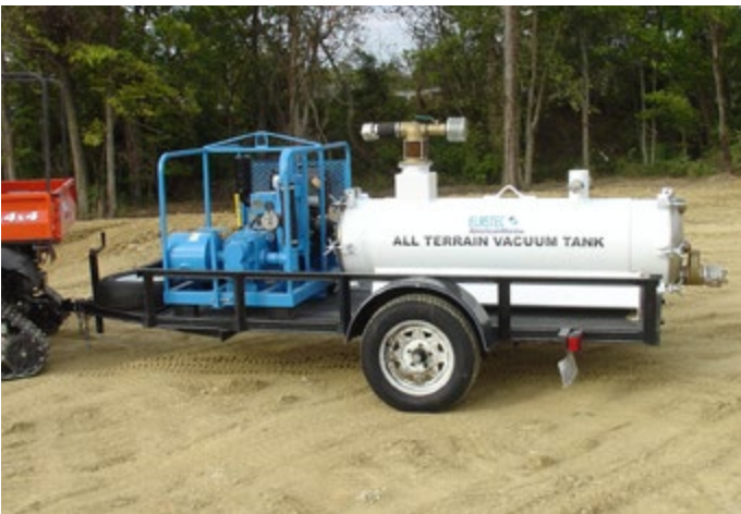
Removable chassis makes trailer transportation easy.
