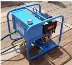
The D9 is a compact and portable diesel-driven hydraulic power unit for operating a boom reel fitted with controls. It features a hand and electric start diesel engine mounted in a steel cage frame. The open style allows excellent access for maintenance.
