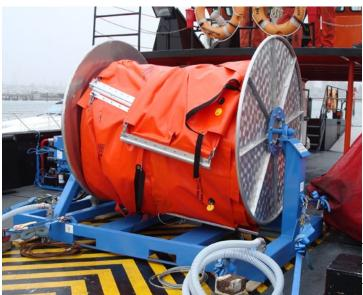
Elastec boom reels are built for safe and controlled deployment and recovery of the boom. The boom reel is hydraulically controlled to assist in the deployment and retrieval.
