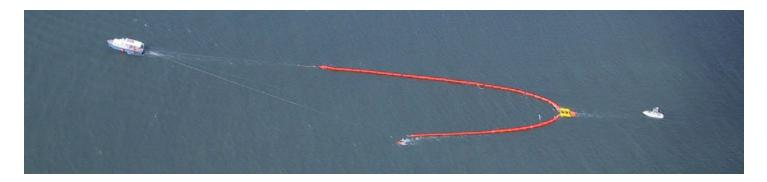
The patented ELASTEC NeatSweep<sup>®</sup> system modernizes the application of oil spill dispersant. The system incoporates a pair of booms that sweep and funnel oil on the surface of the water to the DIspersant Application Zone (DAZ). The towing of the system can be simplified with the addition of an Elastec BoomVane<sup>™</sup>, allowing for a single ship operation.
