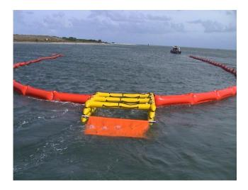
The deflection boom is made up of eight sections of AirMax inflatable oil containment boom, manufactured from high quality Urethane fabric (see next page for spec.)
