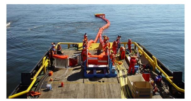
The system includes two sections of AirMax deflection boom, computerized dispersant pumping unit, Dispersant Application Zone (DAZ) and mixing panel, boom reel with air blower, fabric cover and D9 PowerPak.
