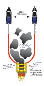
The NeatSweep® system is the most efficient means of applying dispersant chemicals onto an oil slick. The system works by funneling and concentrating the oil on the water's surface before the chemical is applied. Traditional methods spray chemicals onto inconsistent oil layers spread out over water. The result is that dispersant usage can be reduced by up to 50%.
