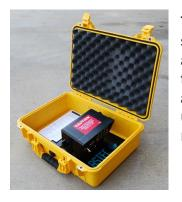
The system includes a control console with manual and automatic setting (that is controlled by speed indicator arm with propeller attached to the ship). The monitor shows the amount of dispersant that is being sprayed and is preset at the factory to control the amount of dispersant (determined by the sweeping width). Since the unit senses the speed of the boat it will increase and decrease flow rate as needed.
