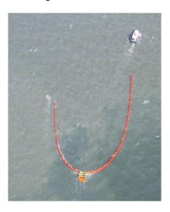
As an option we can supply the NeatSweep® with a Boom Vane so that it may be operated by one vessel.
