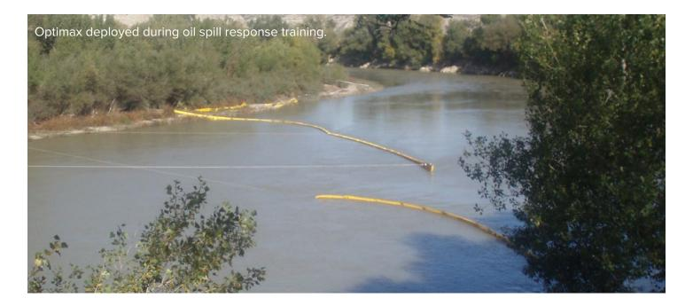
Elastec Optimax booms are comprised of a solid foam log with an added tension member and a skirt. This oil and debris barrier is typically for protected water and fast current use. The top cable and bottom chain give the boom extra strength - holding the boom together even if the fabric becomes damaged.
