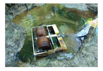
The hydraulic system on this unit will operate Elastec hydraulic trash pumps or high pressure washer or an Elastec Drum Skimmer. The following accessories can be supplied as optional extra;
