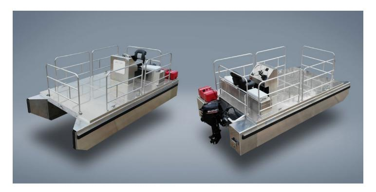
The ELASTEC Catamaran Work Platforms are manufactured at Elastec's Carmi, Illinois USA facility. Its rugged design allows for this versatile catamaran to perform a variety of waterway maintenance and marina tasks. This vessel requires minimal upkeep as it has few moving parts and its propulsion is provided by a single outboard.
