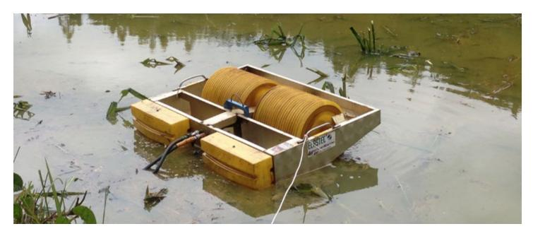
The TDS118 is offered with either the original smooth drums or the latest patented Grooved Drums which can achieve higher oil recovery rates. The Grooved Drum design has been extensively tested by the Ohmsett test facility and researched by the University of California, Santa Barbara. This skimmer has also been independently tested by Environment Canada, CEDRE France, CRREL (Cold Regions Research and Engineering Laboratory). Test reports are available on request.
