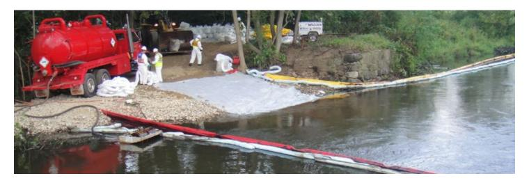
The skimmer can be connected to a vacuum truck to suck out recovered oil. The drums may be driven by the compressed air provided by the trucks braking system.
