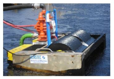
The TDS118 may be supplied with pneumatic or hydraulic motor with a choice of recovered oil pumps - air operated diaphragm or hydraulic driven submersible (E150). The optional diaphragm pump may be remotely positioned or mounted on the skimmer for high head applications.
