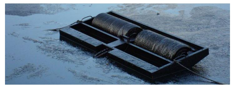
The TDS136 is offered with either the original smooth drums or the latest patented Grooved Drums which can achieve higher oil recovery rates. The Grooved Drum design has been extensively tested by the Ohmsett test facility and researched by the University of California, Santa Barbara. Test reports are available on request.
