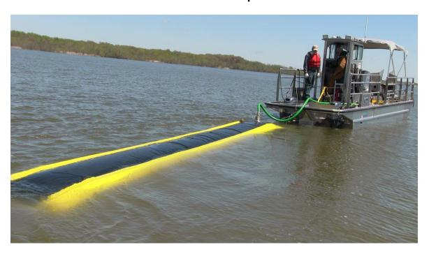
Elastec Towable Bladders are affordable collapsible temporary storage devices that can be used to store recovered oil on dry land or floating in the water. The bladders incorporate tension members running down both sides of the main storage chamber. They also incorporate buoyancy panels fitted with closed cell foam.
