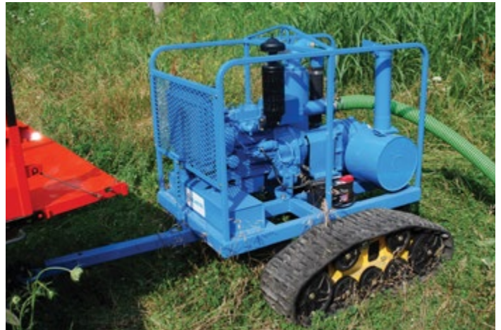
All Terrain Vac features towable ATV chassis.
