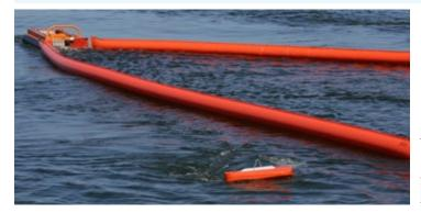
The boom is stored and deployed from a hydraulically operated boom reel with diesel power pack. High capacity diesel driven air blower for boom inflation / deflation. Included with the system is Sweep boom with 100ft / 30m of rugged air-inflatable oil boom, that incorporates the hydraulic and discharge hoses. This single point inflation boom chambers are fitted with foam panels that act as reserve buoyancy and integrated netting assists in retaining the sweep configuration.
