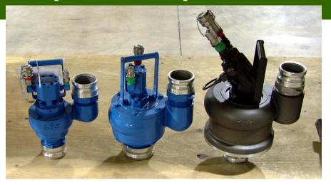
Hydraulic driven submersible pumps – Centrifugal and Helical Screw
